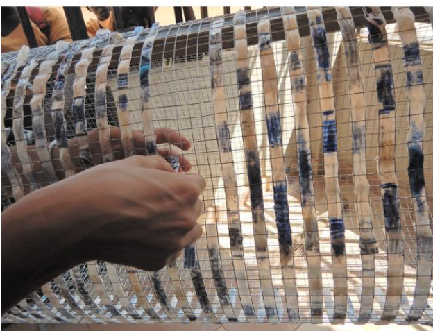
Fig.4. Making of the screens using plastic bags.
